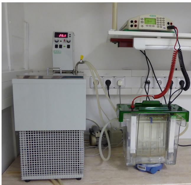
**Figure 1. The setup of the electrophoretic apparatus (lower right corner) with cooling thermostat (left) and power supply (upper right corner)**
