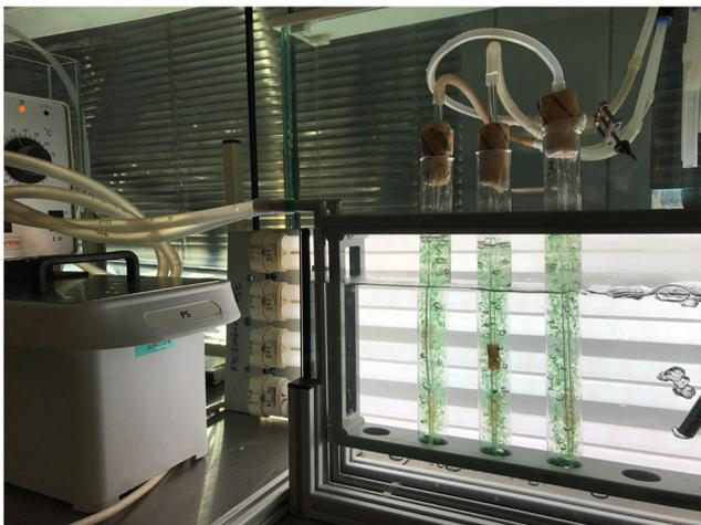
**Fig. 1** Laboratory cultivation unit with side illumination panel fitted with high-frequency fluorescent tubes. Glass 100-mL columns with microalgae cultures are submerged in temperature-controlled water bath
