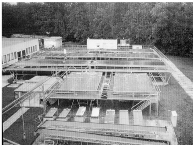
**Fig. 5** In the 1990s, various thin-layer cultivation units with an area from 2 to 225 m<sup>2</sup> were tested. An important improvement was that in the largest units, the system of transversal baffles was replaced with plastic rods (diameter of 13 mm) mounted over a distance of 150 cm perpendicularly to the culture flow. This guaranteed high turbulence due to the flow of suspension under and over the rods with an average layer thickness of about 10–15 mm
