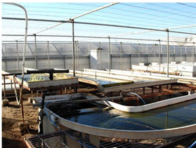
**Fig. 12** Labyrinth-like thin-layer system of 32 m<sup>2</sup> in area with total volume of 1200 L was constructed at the University of Almería, Spain (Morales-Amaral del Mar et al. 2015). The layer thickness of culture is about 20 mm. The culture is pumped from the aerated tank to the first layer using a low-stress centrifugal pump; then it is circulated by gravity at 0.2 m/s until it returns back to the tank
