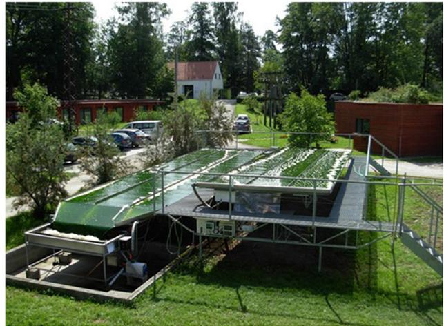
**Fig. 10** Outdoor thin-layer cascade for cultivation of microalgae constructed from stainless steel. It has an area of 90 m<sup>2</sup> and can be operated with a volume between 500 and 1500 L. The surface-to-total-volume ratio can be operated in the range between 60 and 180 1/m corresponding to a layer thickness of suspension between 5 and 15 mm
