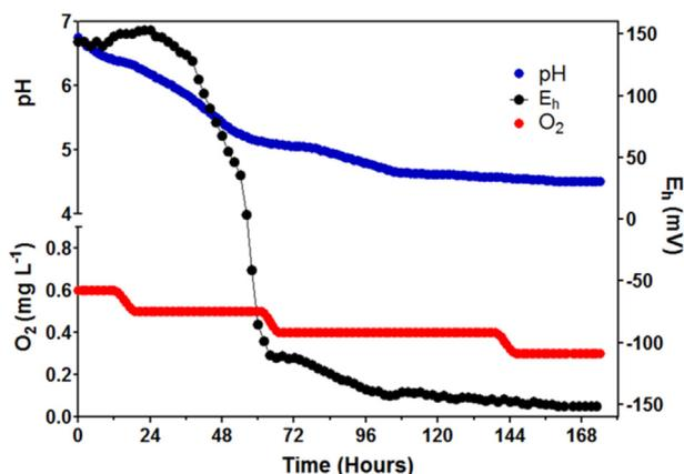
**Fig. 5 –** Time courses in redox potential (E<sub>h</sub>) (black circles), dissolved oxygen (red circles) and pH (blue circles) in the illuminated *Chlorella* cultures during the H<sub>2</sub> production process. (For interpretation of the references to color in this figure legend, the reader is referred to the Web version of this article.)
