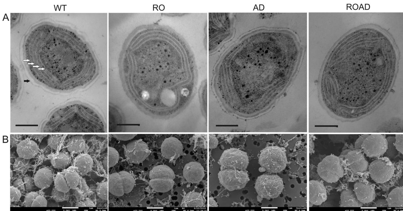
Fig. 1. Electron micrographs of *Synechocystis* wild-type (WT), RO, AD and ROAD cells cultured at  $25^\circ\text{C}$ . (A), TEM micrographs of thin sections. White arrows indicate thylakoid membrane pairs; black arrow shows the S-layer of the cyanobacterial envelope. Bars: 300 nm. (B), SEM images, bars:  $1 \mu\text{m}$ .
