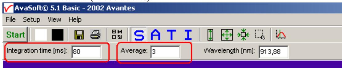
THIS STEP DECIDES ON THE QUALITY OF SPECTRA! SO TRY TO USE AS MUCH OF THE DYNAMIC RANGE OF THE DETECTOR (0-3700 COUNTS) AS POSSIBLE- EXPERIMENT WITH THE INTEGRATION TIME TO GET THE BEST SIGNAL. TOO SHORT TIME MEANS NOISY SIGNAL, TOO LONG CAN OVERSATURATE THE DYNAMIC RANGE. (Of course, you need to have the excitation LEDs on and sample in place when adjusting the sensitivity = see the next paragraph).
