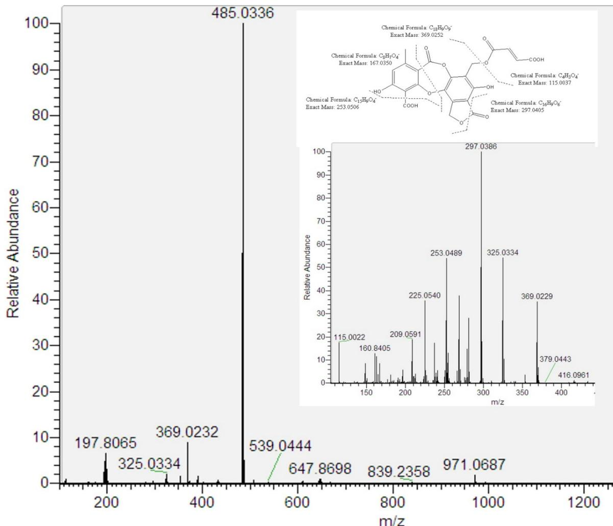
**Figure 3.** ESI/MS/MS spectra of [M-H]<sup>-</sup> of peak 7 and its proposed fragmentation pathway.
